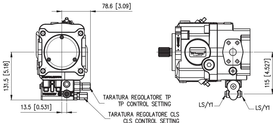
LS: Attacco pressione Load Sensing / Load Sensing Pressure port - 1/8 G (BSPP) Prof./Deep 10 [0.393]
