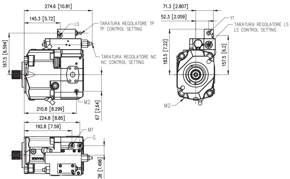
LS: Attacco pressione Load Sensing / Load Sensing Pressure port - 1/8 G (BSPP) Prof./Deep 10 [0.393]
